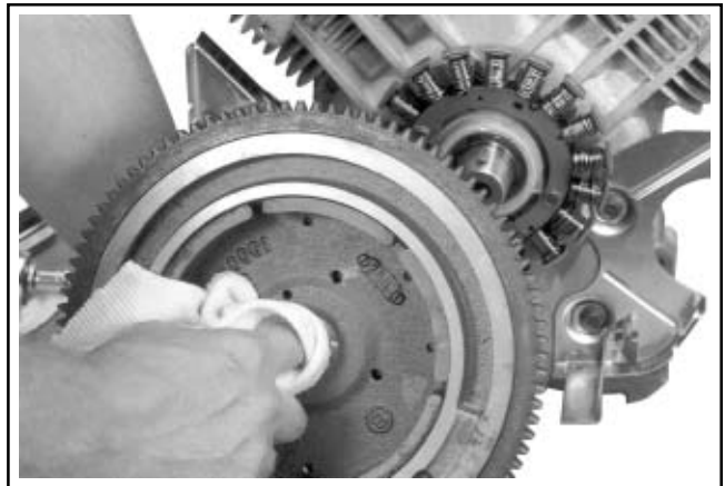
Figure 11-27. Clean and Dry Flywheel Hub.
